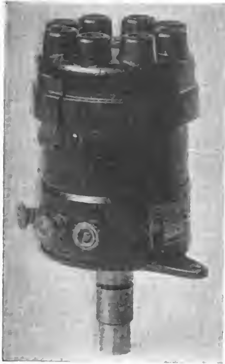
Above—Westinghouse unit comprising breaker, distributor and coil in one assembly. Below—Diagram of Westinghouse breaker. T is the point adjustment and S the locking screw
